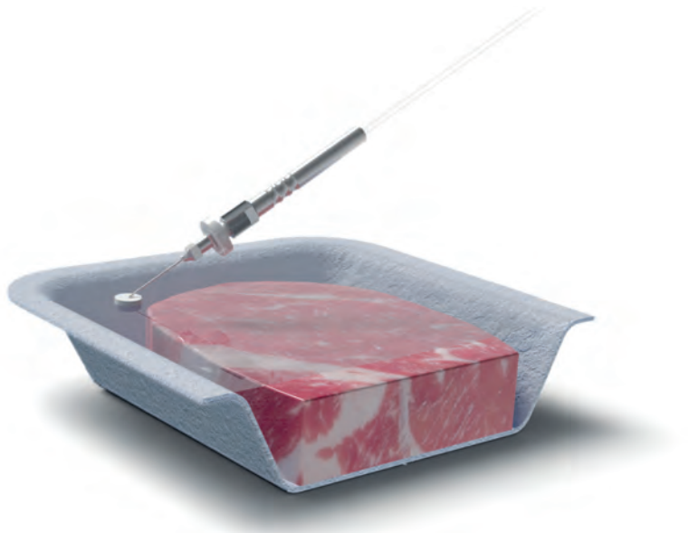
Taking a protective gas mixture sample from a food package
